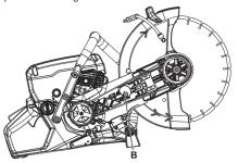
Fit the belt guards and tighten the nuts (A) finger tights. Wiggle the blade guard (E) up and down 3-5 times, and then tighten the nuts (A) with the combination spanner.
