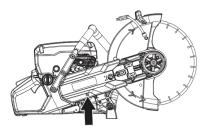
Replace the drive belt. Turn the belt tensioner (B) to position "1" to tighten the drive belt.
