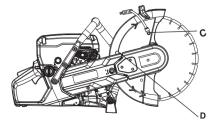
The cutting head is now loose and can be removed from the machine. Remove the belt from the belt pulley.
