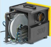
The figure above shows the inside of Trotec's TTR 300 including the desiccant wheel. Even though this industrial desiccant dehumidifier is very compact, it is not suited for typical applications at home due to the missing water collection container.
