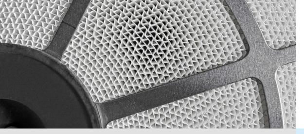
Detailed view of the desiccant wheel of the comfort desiccant dehumidifier TTR 57 E. The rotor is coated with silica gel, a desiccant with a very large hygroscopic surface. In professional industrial desiccant dehumidifiers, each gram of this desiccant has a surface of more than 700 square metres. This means that less than 10 grams have a surface as large as an entire football pitch.
