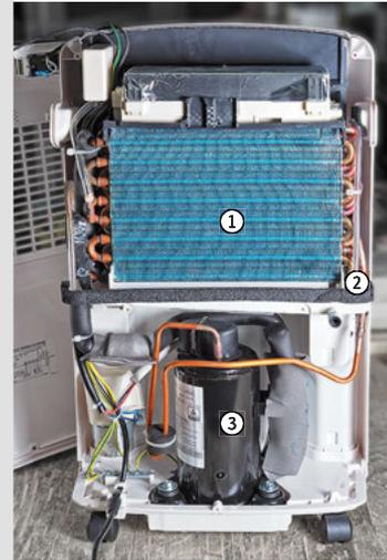
A refrigerant compression dryer opened for servicing shows the heat exchanger integrated in the upper part of the device with the evaporator (1) at the front, on the cold surface of which the air condenses, and the channel (2) behind it serving to discharge the accumulated condensate into the water collection container. The compressor (3) for the refrigerant is integrated in the bottom part of the device.
