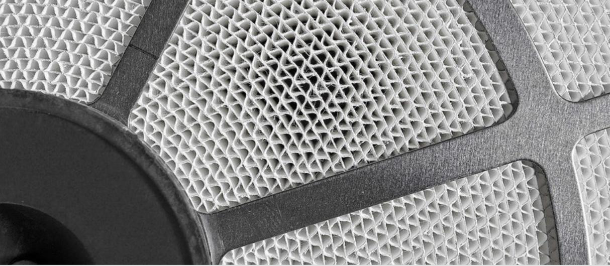
Detailed view of the desiccant wheel of the comfort desiccant dehumidifier TTR 57 E. The rotor is coated with silica gel, a desiccant with a very large hygroscopic surface. In professional industrial desiccant dehumidifiers, each gram of this desiccant has a surface of more than 700 square metres. This means that less than 10 grams have a surface as large as an entire football pitch.
